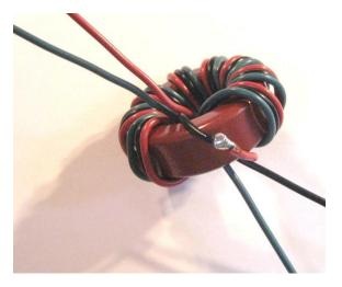
Trim and strip the remaining *right green* wire at about 2". Cut an additional 2" piece of green wire, and crimp and solder both wires to a # 8 lug. The 2" green wire will connect to the ground
